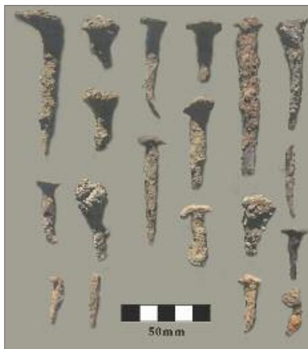
Pl. X.1 Iron nails and rivets from High Medieval Phases 1–2.
